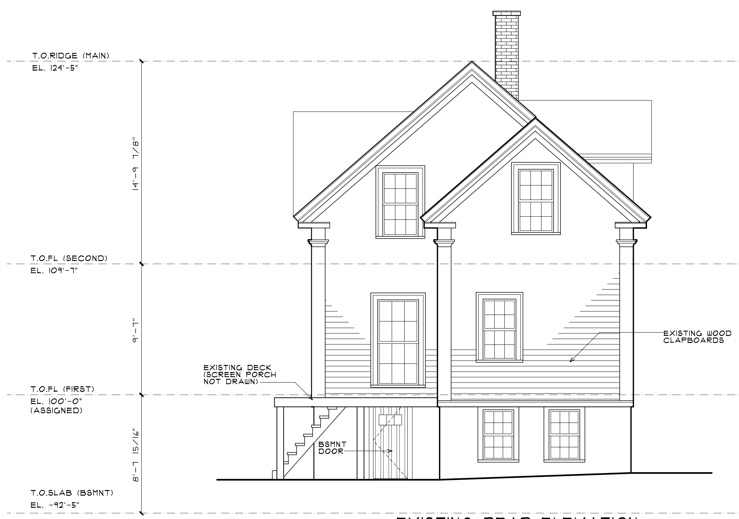
EXISTING REAR ELEVATION SCALE: 1/4" = 1'-0"
